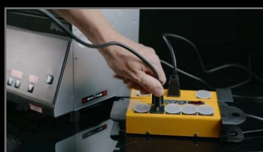
PLUG THE VACCUM CLEANER CORD IN THE "VACUUM" SLOT, AND TURN IT ON (OPTIONAL)
